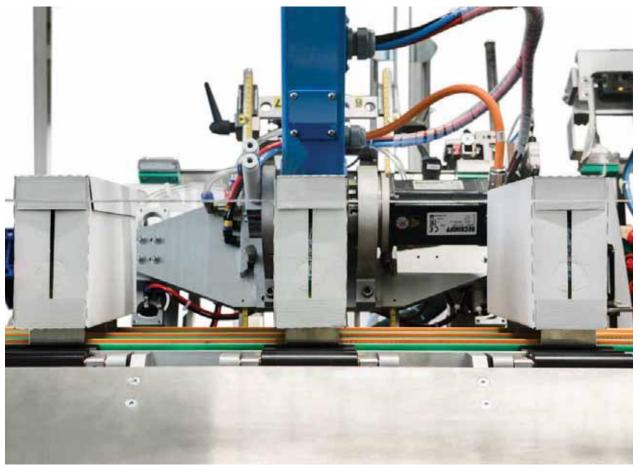
keep the pouches horizontal, filling the case up to its outer edge, since the front side of the case remains open until the filling is completed.
